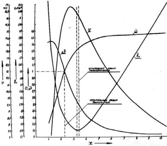
Fig.3. The dependence of non-dimensional expense  $\varpi$  on non-dimensional edge step  $x$ .
