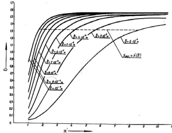
Fig.4. The dependences  $\varpi$ ,  $v$ ,  $\Delta \bar{P}$ , and  $\bar{R}_T$ , realizing in air heat exchanger, on non-dimensional edge step  $x$ .
