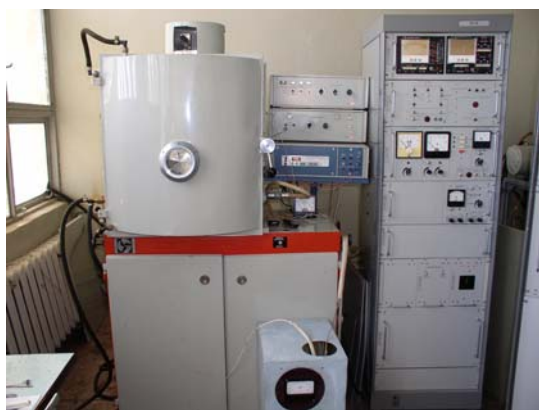
Fig.1. Vacuum plant VU-1 with the system of ionic etching.
