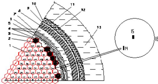
Fig.3: Configuration of reactor core and crystallography section. 1- Reactor core; 2- Cladding fuel Assembly; 3- Core baffle; 4- Water; 5- Basket; 6- Core barrel; 7- Shield; 8- Pressure vessel; 9- air gap; 10- Cladding; 11- Thermal insulation; 12- Tank wall; 13- Biological shield; 14- Crystal monochromator; 15- Metallic sphere.
