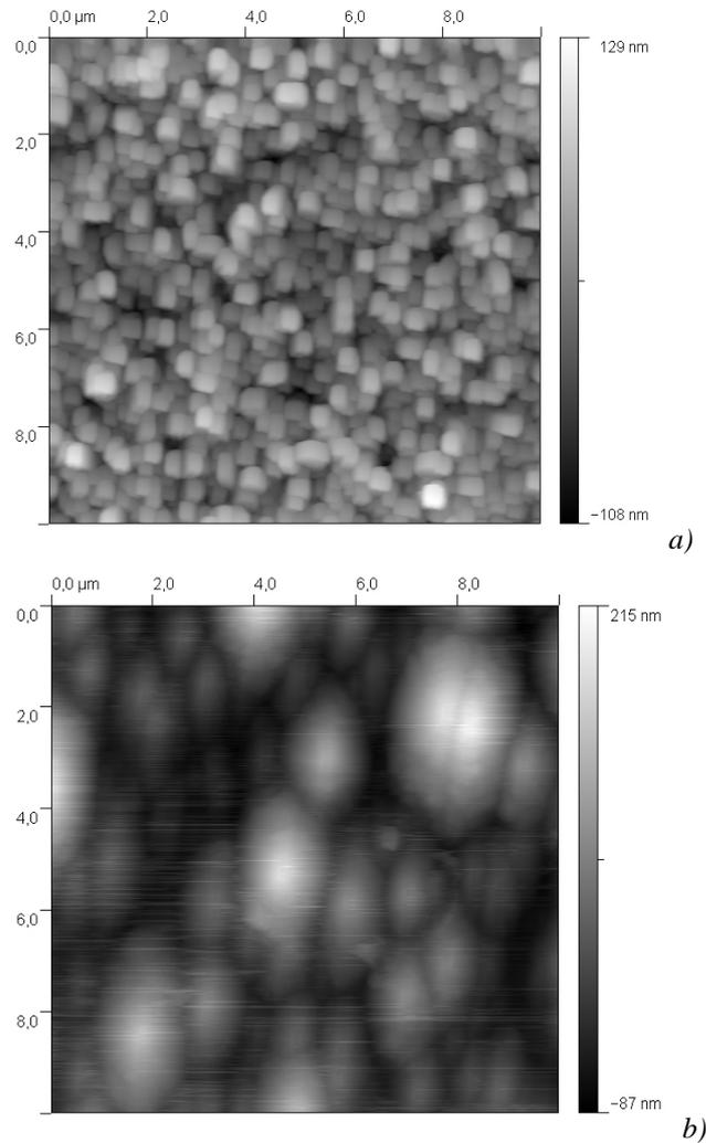
Fig. 2. AFM images of GaInPN layers on (a) silicon substrate, (b) gallium arsenide substrate.
