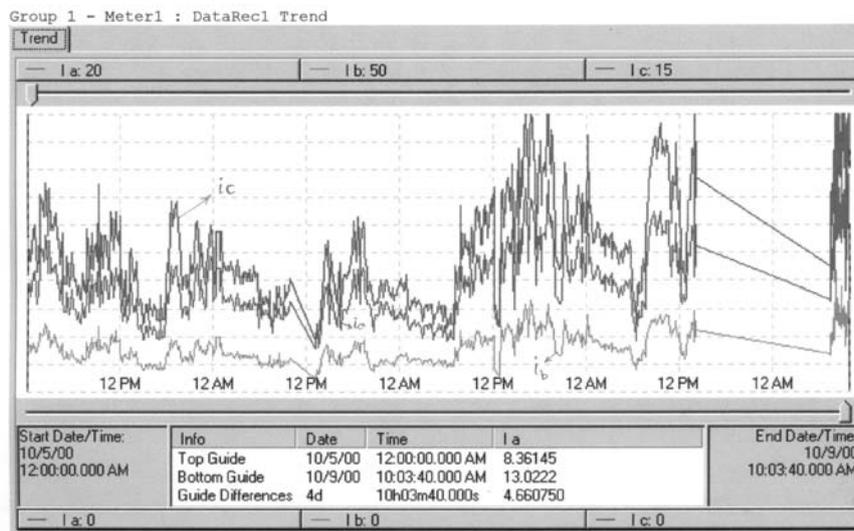
**Fig (4-d): Load side currents vs. time.**
