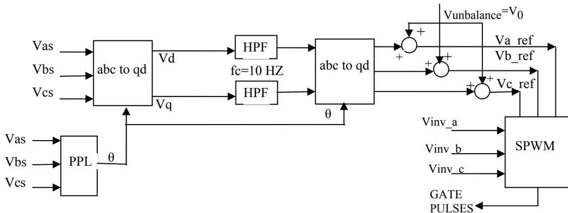
Fig (6): Control block diagram of SAF.
