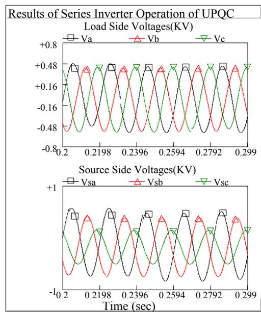
**Fig (10): Simulation results of series part of UPQC.**
