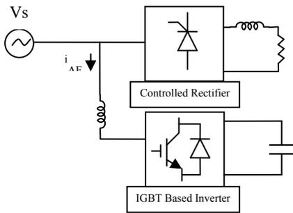
Fig (1): Single line diagram of PAF.
