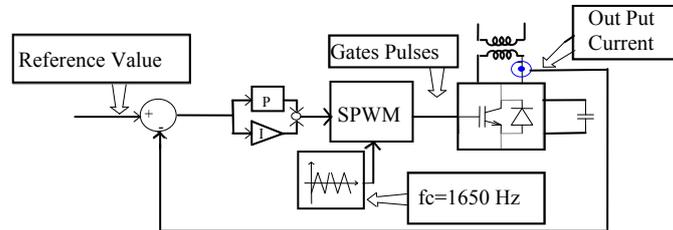
**Fig (7): SPWM generating circuit.**
