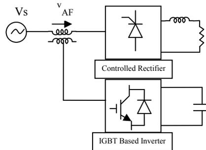
Fig (2): Single line diagram of SAF
