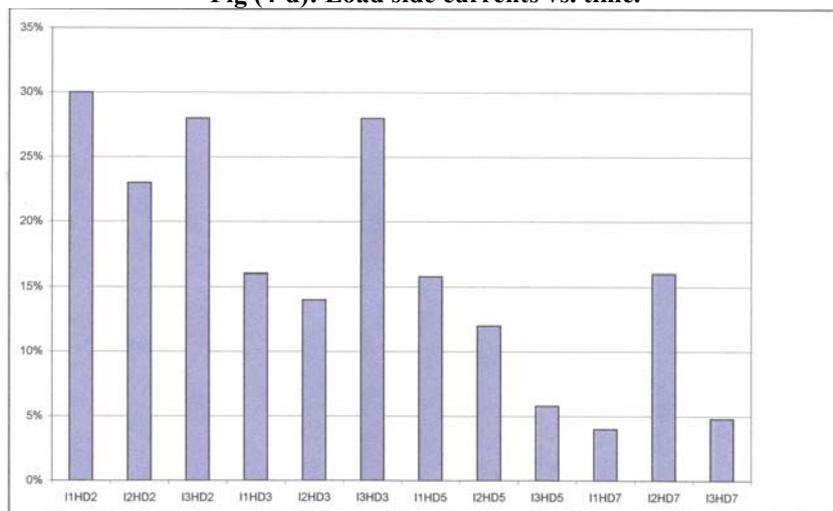
**Fig (4-e): Harmonic spectrum of load side currents.**
