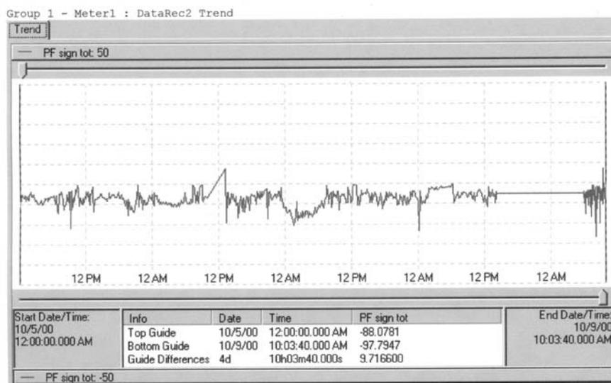
**Fig (4-b): Power factor vs. time.**
