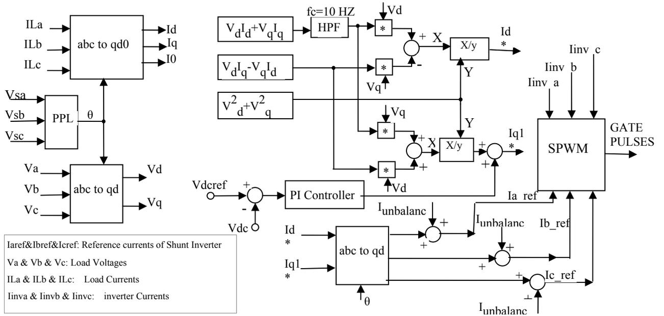
Fig (5): Control bloke diagram of PAF.
