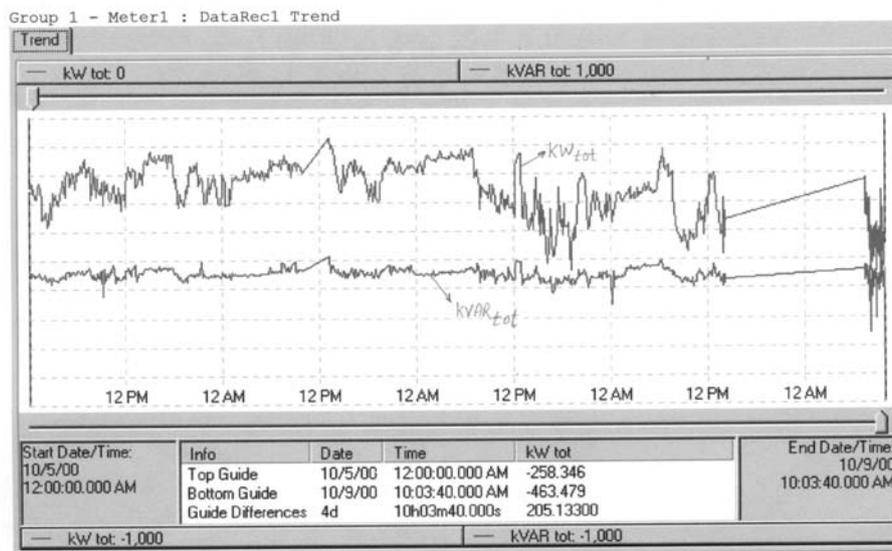
**Fig (4-a): Total active and reactive power vs. time.**
