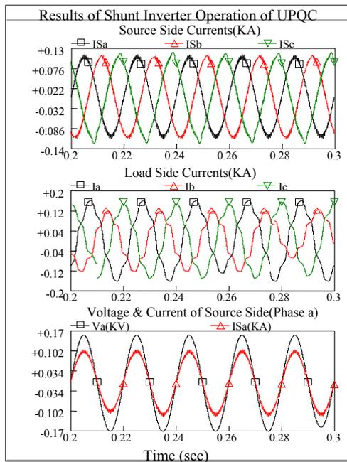
**Fig (9): Simulation results of shunt part of UPQC.**
