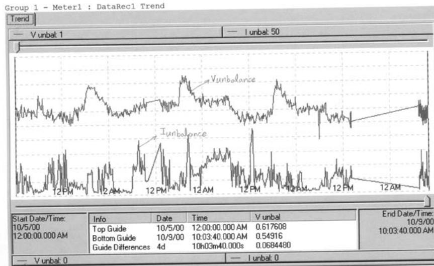
**Fig (4-c): Voltage imbalance and current imbalance vs. time.**
