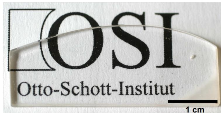
**Figure 6.1:** Transparent  $BaF_2$  nanocrystal containing glass ceramics [10].
