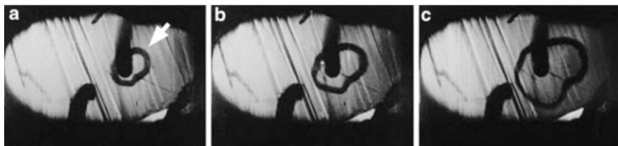
Fig. A.13 Ring-shaped high-field domain ( arrow ) enclosing a small circular cathode and expanding ( a )–( c ) in time (pictures taken in 1 s time intervals). After the high-field domain touches the anode at the end of the contact wire at the lower middle left, the ring disappears, a new ring develops at the cathode, and the cycle repeats itself (period length 5 s, contact distance \sim 2 mm).
