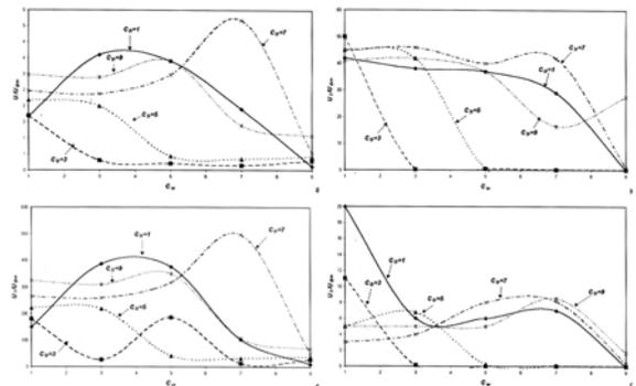
Fig.1.4. Calculated curves of the overvoltage in case of the steady regime and its harmonic components respect to nominal voltage: a – orders of the overvoltages, b – 3rd harmonics, c – 5th harmonics, d – 7th harmonics
