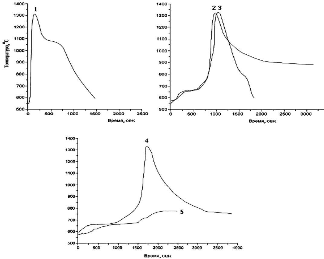
Figure 3. The synthesis thermograms at different temperature values of the reactor's wall. 1 –  $T_0 = 1050^\circ\text{C}$  (the disconnection of the source was made in the moment of reaching maximum temperature by the reacting mixture). 2, 3 –  $T_0 = 850^\circ\text{C}$  (Thermogram 3 – synthesis with the disconnection), 4 –  $T_0 = 750^\circ\text{C}$ , 5 –  $T_0 = 730^\circ\text{C}$
