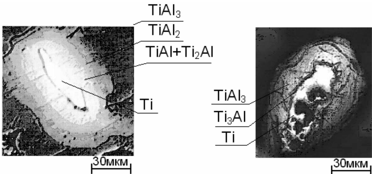
Figure 4. The photos of typical elements of the structure, corresponding to the modes 1 and 3 (Fig. 3)
