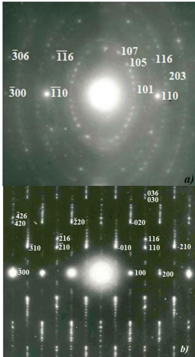
*Fig. 1.* Rotation electron diffraction pattern of the CdInGaS<sub>4</sub> single-crystal thin films: a) electron diffraction patterns imitating electron diffraction patterns of lamellar texture. b) electron diffraction patterns imitating electron diffraction patterns of acicular texture.
