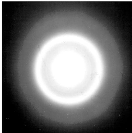
Fig. 1. Electron diffraction patterns of TlGa<sub>0.96</sub>Ge<sub>0.04</sub>Se<sub>2</sub> amorphous film.
