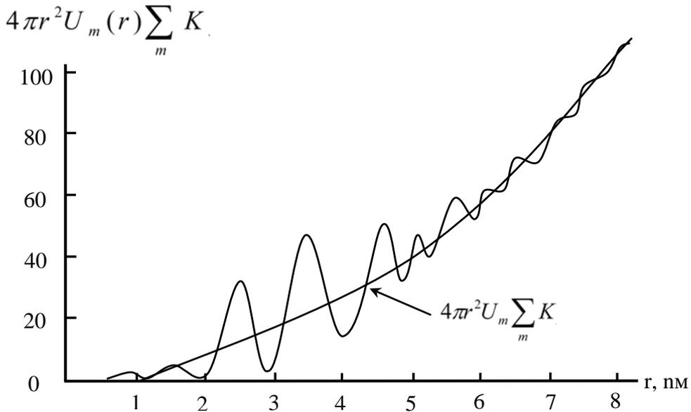
Fig. 3. Radial distribution curve of TlGa<sub>0.96</sub>Ge<sub>0.04</sub>Se<sub>2</sub> atoms.
