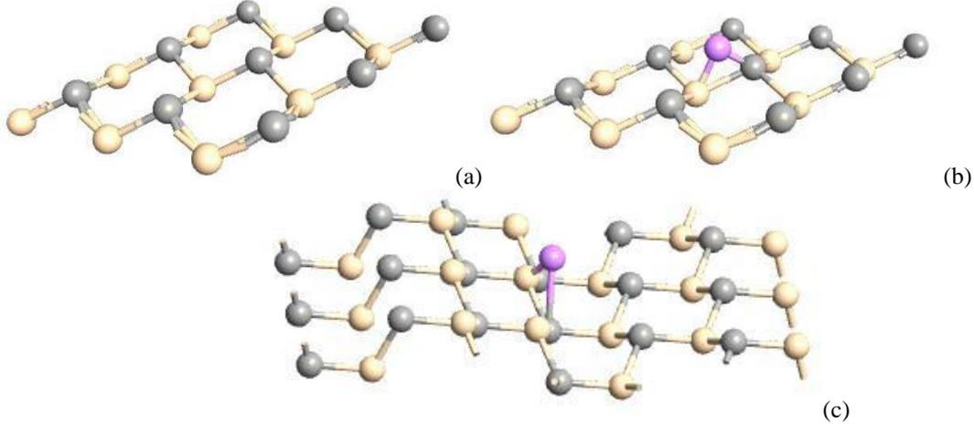
Fig.1. Atomic structure of (a) pristine cubic  $2 \times 1$  SiC, (b) Li adsorbed on face centered cubic  $2 \times 1$  SiC, (c) Li adsorbed on hexagonal  $3 \times 1$  SiC.
