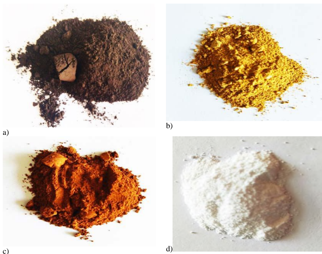
Fig.2. Photographs of a)CuO, b)CuAl 2 O 4 (12% Cu), c)CuAl 2 O 4 (25% Cu) and d)γ-Al 2 O 3 crystals.
