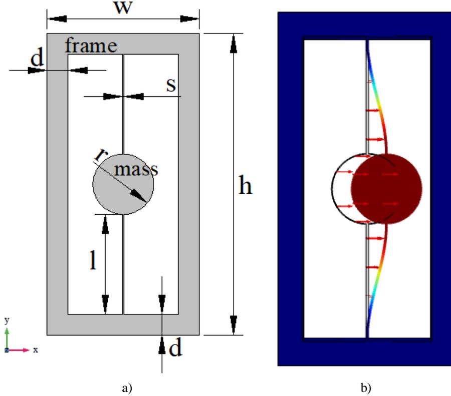
Fig. 1. a) Unit cell of a metamaterial with nonlinear local resonance b) resonance mode of the 3D unit cell (416.89 MHz)
