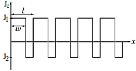
Fig. 2. Critical current density dependence in long junction with  $N=5$
