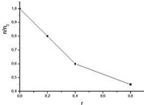
Fig.3. Power exponent  $n$  in I-V curve of granulated superconductor using long junction limit in respect to short junction limit  $n_0$  versus geometrical factor.
