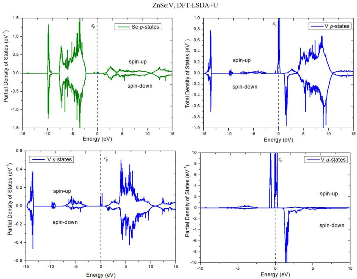
Fig. 4. Partial DOS for  $Zn_{15}V_1Se_{16}$  with LSDA+U.
