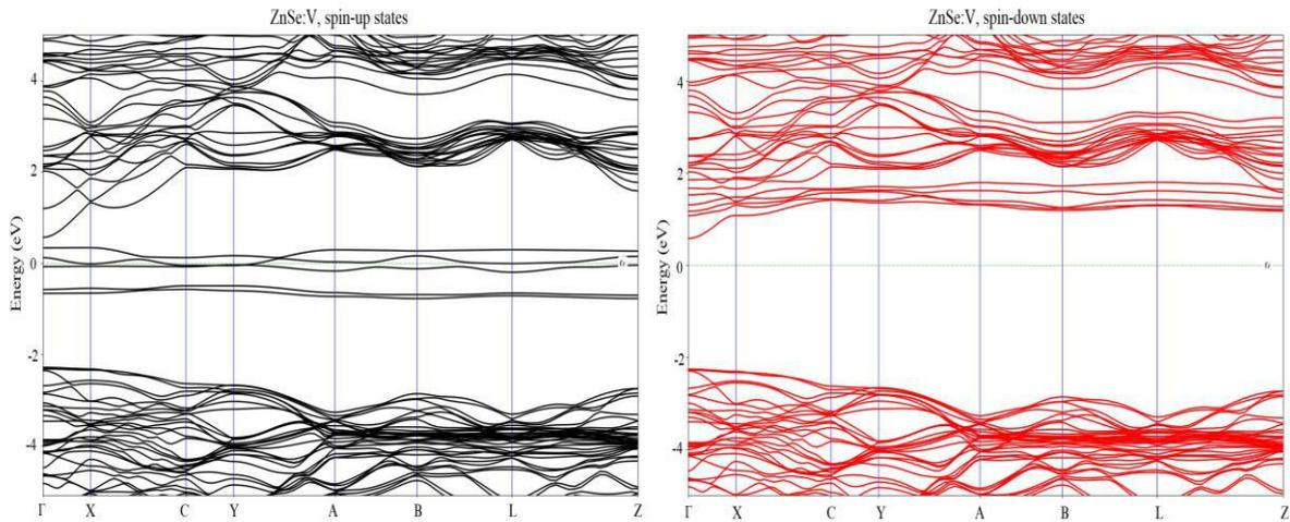
Fig. 2. Spin-polarized band structures for  $Zn_{15}V_1Se_{16}$  correspondingly to spin-up and spin-down states.
