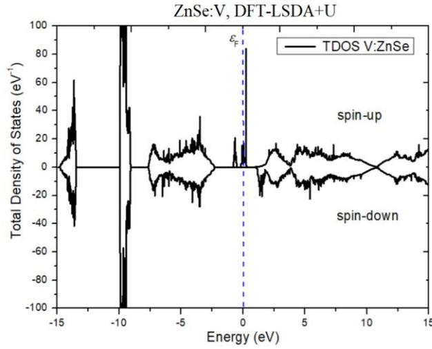
Fig. 3. Total DOS for  $Zn_{15}V_1Se_{16}$  with LSDA+U.
