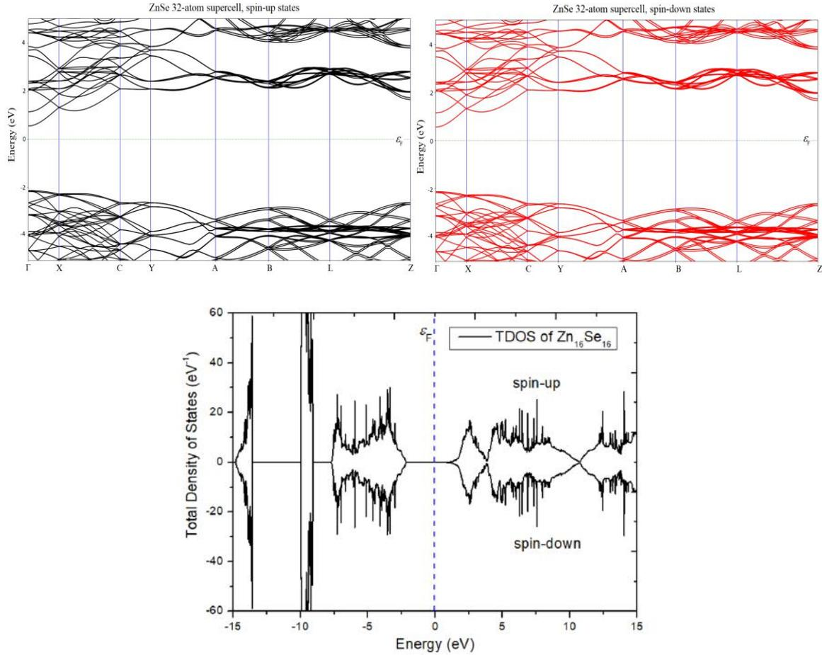
Fig.1. Spin-polarized band structures and TDOS for  $Zn_{16}Se_{16}$  correspondingly to spin-up and spin-down states .
