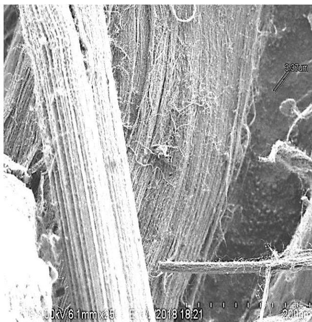
Fig. 1 – SEM image of synthesized MWNTs
