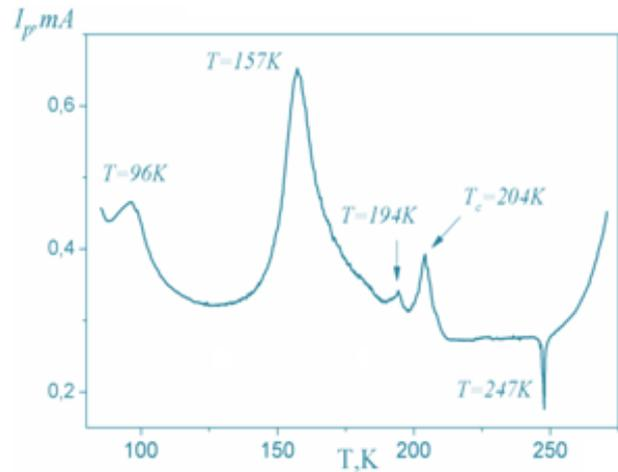
Fig. 4. - Temperature dependence of the pyroelectric current generated in TIInS<sub>2</sub>:La after sample poling at  $\sim 77$  K by dc electric field  $\sim 5$  kV/cm. The heating rate was 20 K / min.
