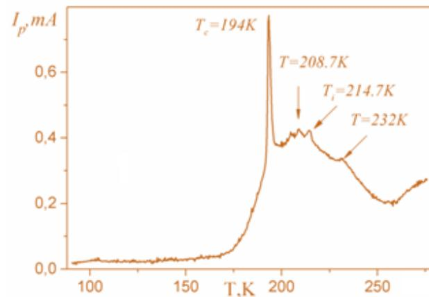
Fig. 5. - Temperature dependence of the pyrocurrent generated in TIInS<sub>2</sub>:La after sample poling by dc electric field  $\sim 5$  kV/cm in the temperature region  $\sim 210 - 300\text{K}$  in cooling . The heating rate was 20 K / min.
