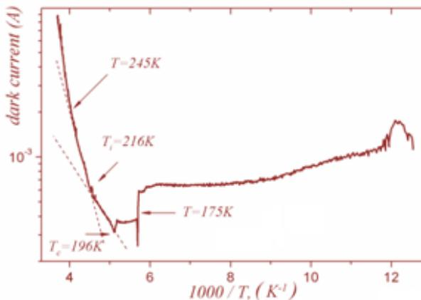
Fig. 9. - Dark current versus temperature for TlInS<sub>2</sub>:La shown in the Arrhenius plot. The measurement was carried out in the direction parallel to the layer at the bias of ~ 10V. The heating rate is 2 K min<sup>-1</sup>.
