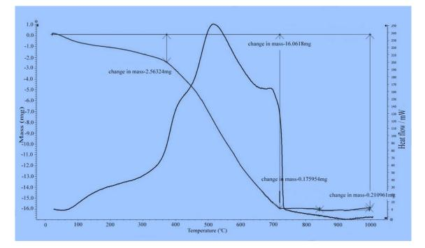
Fig. 4. TGA/DSC analysis of f-MWCNTs
