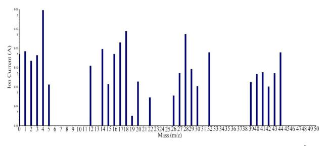
Fig.8. Mass spectrum of gaseous products of the oxidation-thermal decomposition process of the f- MWCNTs at 500 °C
