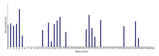
Fig.10. Mass spectrum of gaseous products of the oxidation-thermal decomposition process of the f - MWCNTs sample at 600°C.
