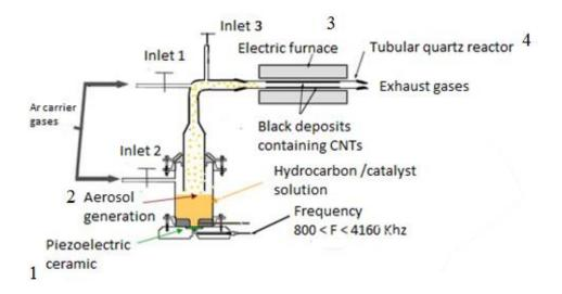
Fig.1. Schematic diagram of ACVD apparatus.
