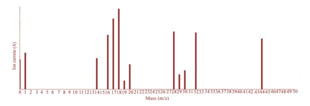
Fig. 6. Mass spectrum of gaseous products of the oxidation-thermal destruction process of the f - MWCNTs sample at 370 °C.
