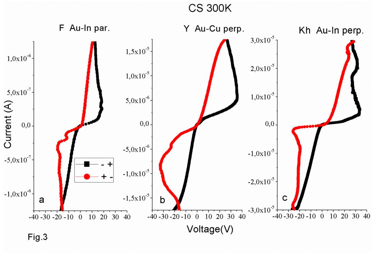
Fig. 3. The Pinched hysteresis loops registered for three different  $TiGaSe_2$  samples by current sweep method at 300 K.
