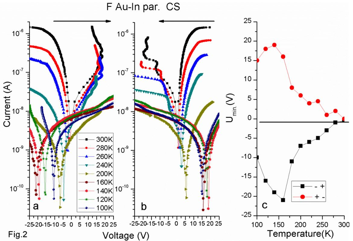
Fig. 2. a) and b)  $I - V$  characteristics of  $F$ -type TlGaSe<sub>2</sub> sample with  $Au - In$  metallic electrodes deposited on the top surface of crystal parallel to the layers. The measurements were carry out in current sweep method.  $I - V$  characteristics are displayed in logarithmic scale and corresponded to different temperatures. Arrows indicate the direction of sweep; c) The temperature dependences of "beak" position in Fig. 2 (a and b) for different direction of sweep.
