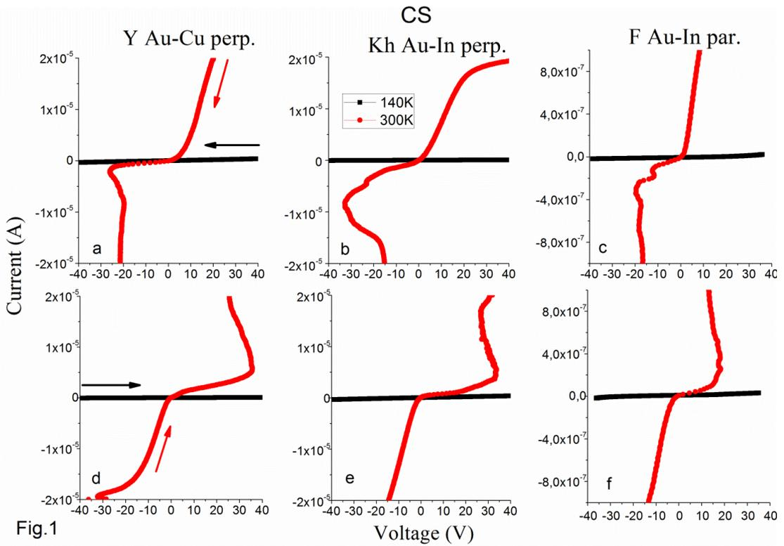
Fig. 1.  $I - V$  characteristics of different TlGaSe<sub>2</sub> samples measured by current sweep method in linear scale at two different temperatures; 140 and 300 K. Arrows indicate the direction of sweep.
