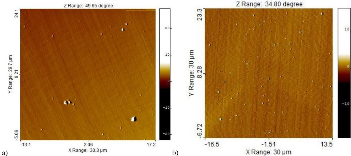
Fig. 3. Atomic force microscopy scans of structures. Morphology and surface defects of semipolar GaN template (left) and InGaN/GaN MQWs heterostructures (right) on  $30 \times 30\mu\text{m}^2$  surface area.
