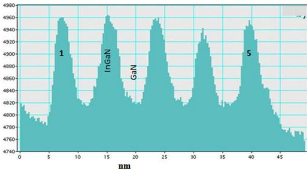
Fig. 5. HAADF image: Intensity profile from bottom to top of the QWs structure along the arrow in numbers help to establish the link between image and profile.
