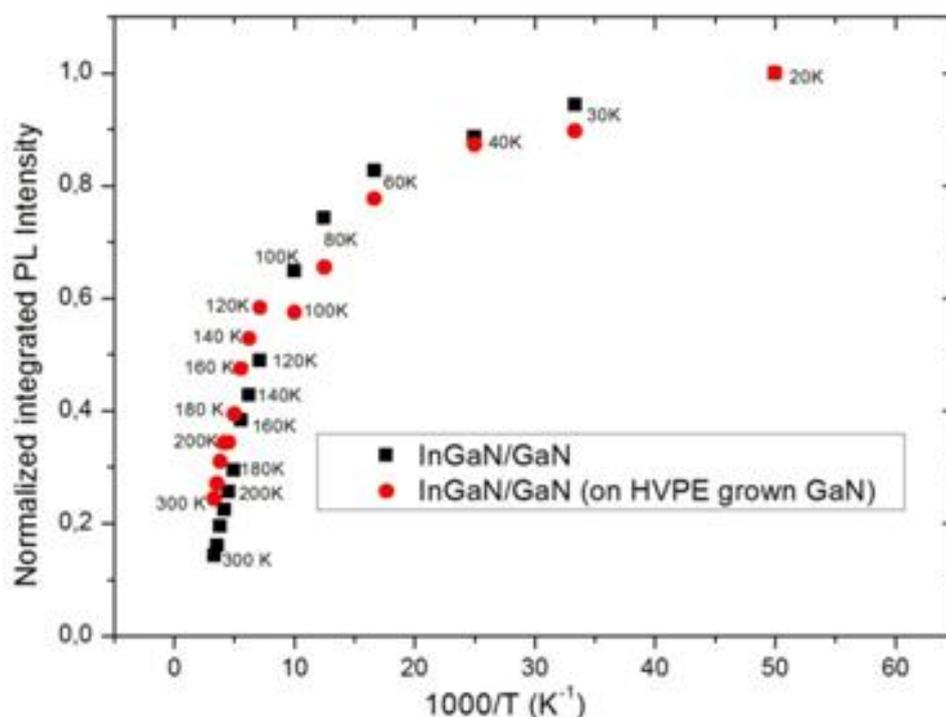
Fig. 8. Arrhenius plot of the normalized integrated PL intensity of InGaN MQWs samples.
