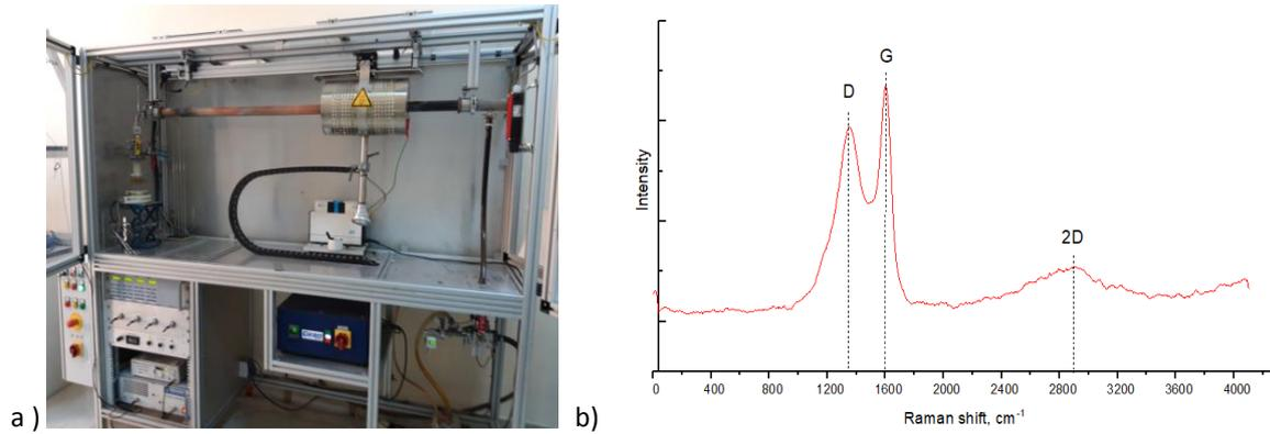
Fig. 1. A-CVD system and Raman characterization of MWCNTs.
