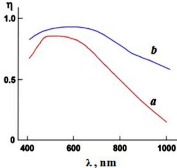
Fig.1. The spectral distribution of EPh layer quantum yield on CdInGaS<sub>4</sub> base without Au impurity (a) and with it (b).
