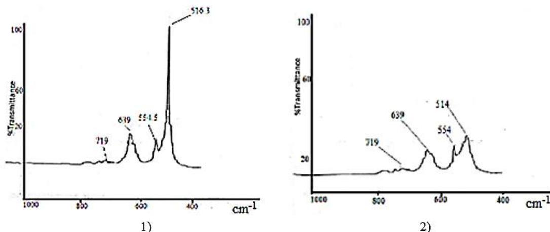
Fig.4. IR-absorption spectra in region 400 – 1000 $\text{cm}^{-1}$  of PTFE/CdS samples after 6<sup>th</sup> cycle of nano-CdS implantation.
