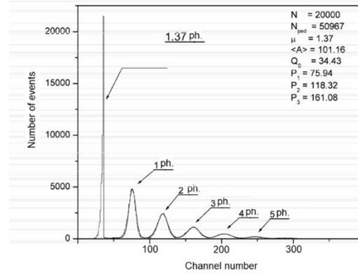
Fig. 3. MAPD spectrum (at fixed T and  $U_{bias}$ ). Designations:  $N$ ,  $N_{ped}$  - respectively the total number of events and the number of events in the pedestal;  $\mu$  is the average number of photoelectrons;  $\langle A \rangle$  - average value of the histogram;  $Q_0$  is the position of the pedestal,  $P_1$ ,  $P_2$ ,  $P_3$  are the positions of the peaks of the 1st, 2nd and 3rd photoelectrons, respectively.
