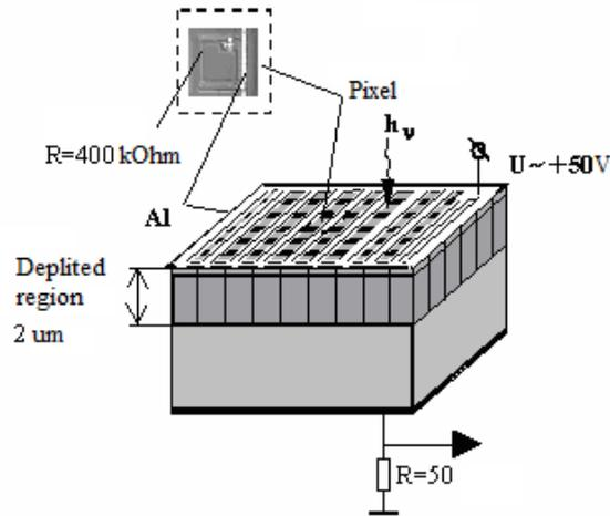
Fig. 1. Schematic view of MAPD photodiode.
