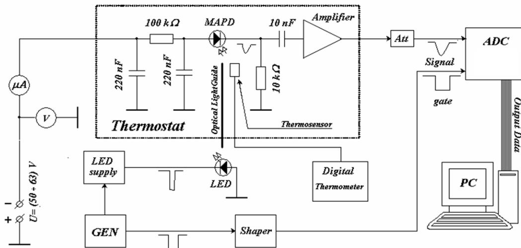
Fig. 2. Experimental setup.
