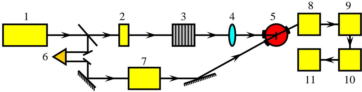
Fig. 1. Schematic of an experimental setup for measuring the transmission spectra of InSe crystals: 1-YAG: Nd<sup>3</sup> laser, 2-crystal KDR, 3-optical filters, 4-lens, 5-sample, 6- delay time, 7-cell with heavy water (deuterioxide), 8-monochromator, 9-detector, 10-oscilloscope, 11-computer system.
