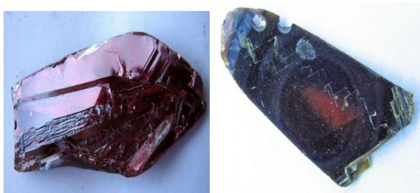
Fig. 1. Single crystals grown by the Bridgman method: TlGaSe 2 on the left, TlGa 0.995 Er 0.005 Se 2 on the right.
