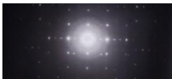
Fig.4 Electron diffraction pattern from single crystal superstructure phase of YbAs 4 S 7 .
