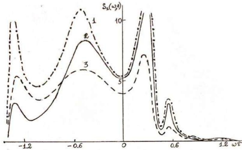
Fig. 2. The reduced spectral density  $S_1(\omega, z)$  of a signal wave as a function of phase modulation parameter  $\omega\tau$  for  $z/l_{nl} = 0,7$  (curves 1 and 2) and  $z/l_{nl} = 1$  (curve 3),  $p = 0$  (curve 2),  $p = 5$  (curves 1 and 3) and  $\Delta = 0, \delta_i = 0$
