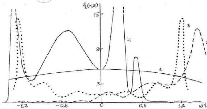
Fig. 3. The reduced spectral density  $S_1(\omega, z)$  of a signal wave versus phase modulation parameter  $\omega\tau$  for  $p = 5, z/l_{nl} = 0,5, \Delta = 0, \delta_i = 0$ ; 1 -  $l_{nl}/l_v = l_{nl}/l_d = 3$ ; 2 -  $l_{nl}/l_v = 0, l_{nl}/l_d = 3$ ; 3 -  $l_{nl}/l_v = 3, l_{nl}/l_d = 0$ ;
