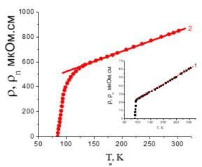
*Fig. 1.* Temperature dependences of the resistivity of the samples: 1- YBa<sub>2</sub>Cu<sub>3</sub>O<sub>7-δ</sub>,
