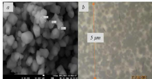
Fig. 1. a) SEM photography of 300 nm sized barium titanate powder; b) micrograph of 300 nm sized barium titanate – oleic acid mixture in optic microscope equipped with high resolution camera.
