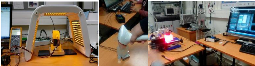
Fig. 1. (a) Laser, b) IPL, and (c) LED devices used in the temperature measurement experiments.
