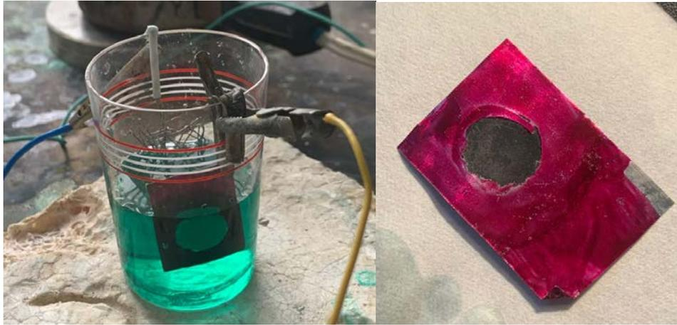
Fig. 4. View of electrochemical cell taken during deposition of Ni (left ) and sample upon deposition (right).
