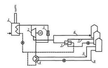
*Fig.* 2. The principal scheme of supply of heating-manufactural boiler rooms by electro generating plants: 1 is steam boiler; 2 is steam turbine; 3 is reduction cooling plant; 4 is condenser; 5 is means water heat exchanger; 6 is steam on technological wastes; 7 is means water, 8 is process water; 9 is heated process water.
