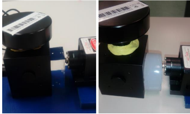
Fig. 1. A picture of the Zerdine (left) and Agar (right) phantoms under test.
