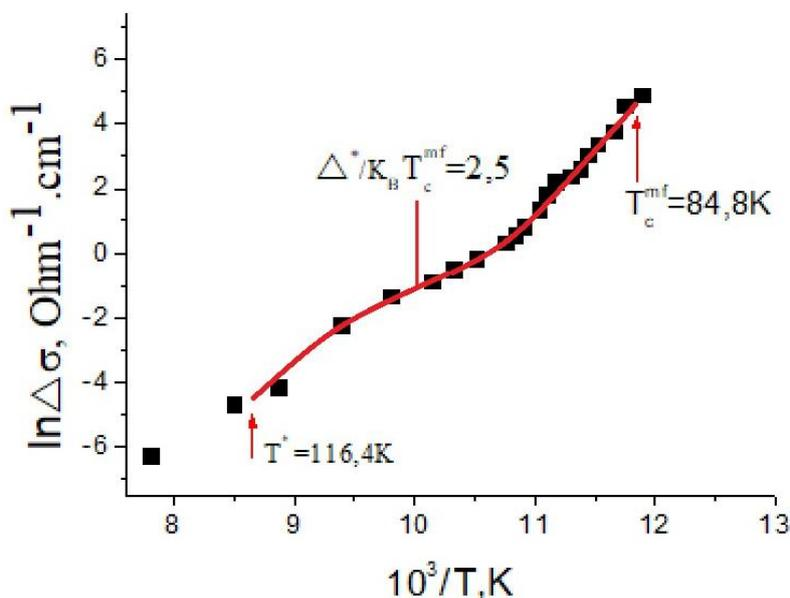
Fig.2. Dependence of the logarithm of excess conductivity on its inverse temperature  $Y_{0.3}Cd_{0.7}Ba_2Cu_3O_{7-\delta}$ , solid lines – approximation level 1 with the parameters given in the text.
