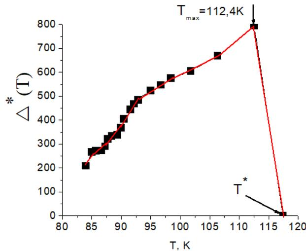
Fig.1. Temperature dependence of the calculated pseudogap value of the sample Y<sub>0,3</sub>Cd<sub>0,7</sub>Ba<sub>2</sub>Cu<sub>3</sub>O<sub>7-δ</sub> with parameters given in the text. Arrows show the maximum values of the pseudogap value.
