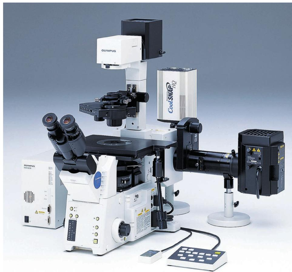
**Figure 2:** The Olympus IX2-DSU confocal system offers a patent-pending spinning slit disk that delivers Nipkow-like optical sectioning with much higher transmission rates.
